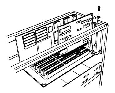
Once the connectors reach the slot, push the card in firmly (but carefully) to insert it fully. You should feel it fit into place. If the card does not go in smoothly, do not force it; pull it all the way out and try again.
